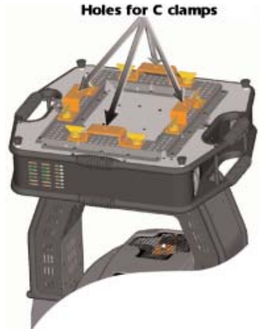
Figure W5 showing clamps fitted
