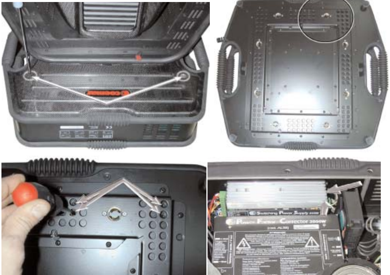
Figure W11A Removing Switching Supply
